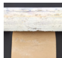
Al-brass tube with seawater fouling
